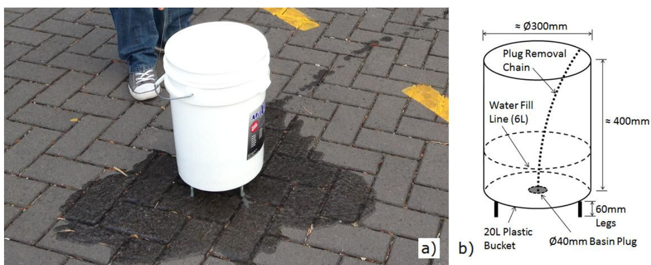
Figure 3. Stormwater infiltration field test (SWIFT) Infiltrometer used in this study. (a) SWIFT in use; (b) SWIFT dimensions.
