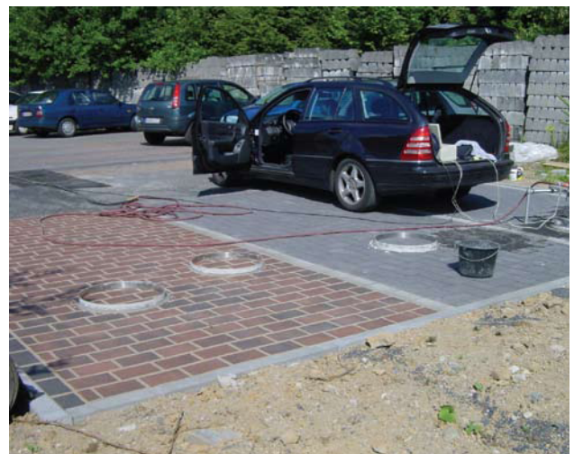
Monitoring the long-term infiltration performance of permeable paving (summarised in the graph below).
